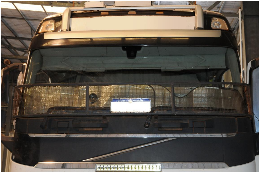
Truck with non-original sun visor fitted at base of window.
